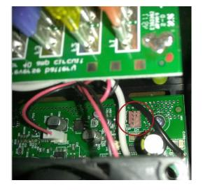
Disconnect it and place a .1 spacing jumper over the 2 pins as shown.
