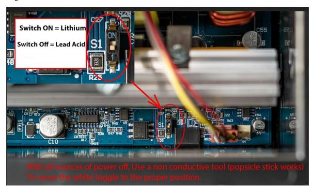
The converter replacement section PD4135CSV, will have the above switch.
